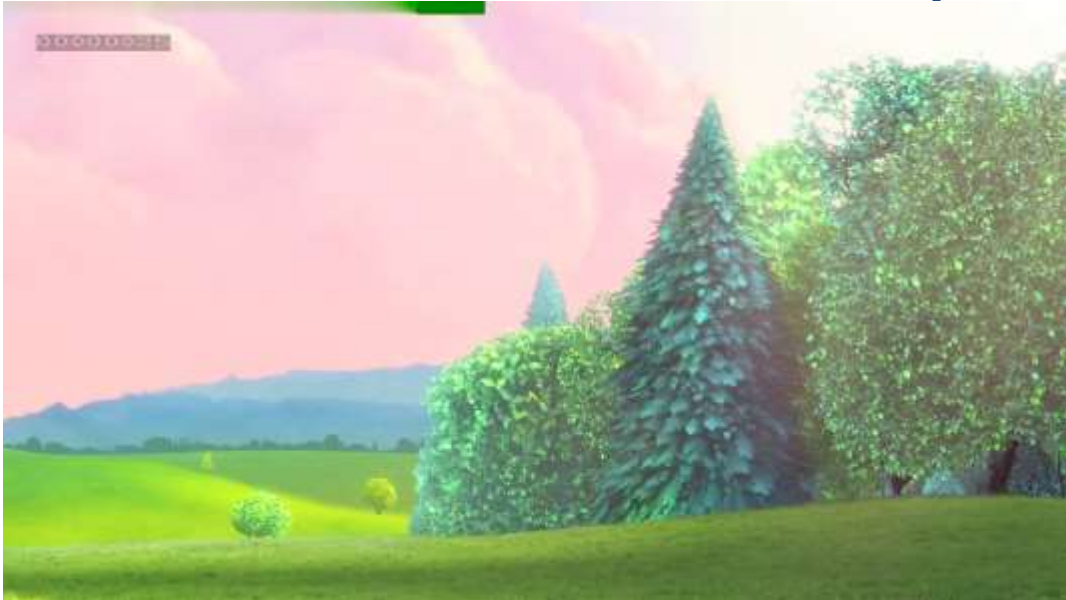
Fig. 4: 1 MNALU of type I (its size is 16x 80 pixels) is overlaid at the position 31 (in Macroblock units)
